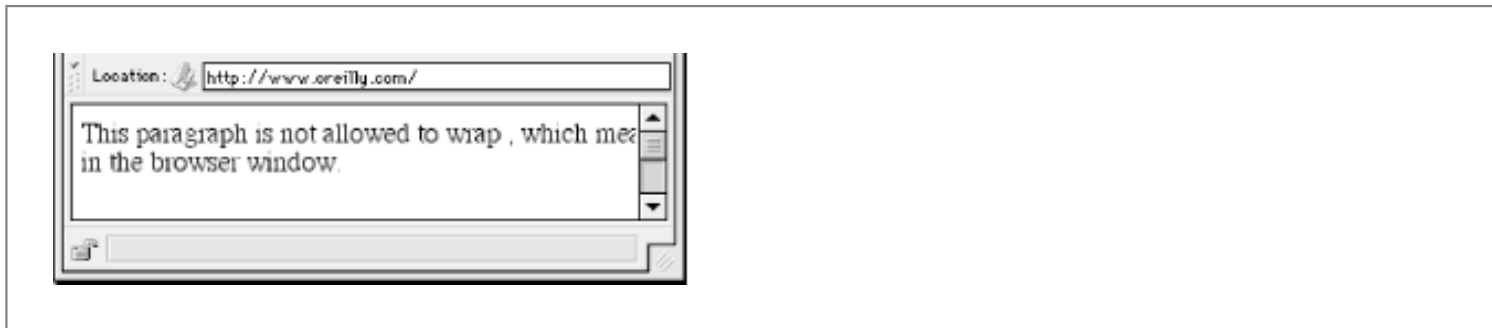
Figure 4-21. Suppressing text-wrapping with the white-space property
