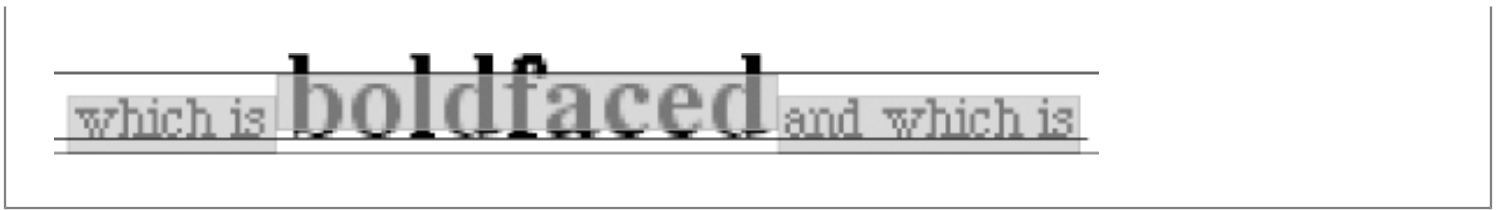
Figure 8-50. How the inline boxes (gray) influence the height of the line box
